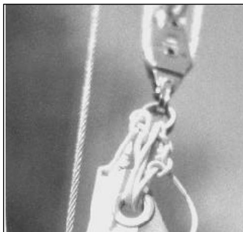
**Take the jib block at the bottom of the mast and fix it to the head of the jib. The small line on the jib is a further security.**
