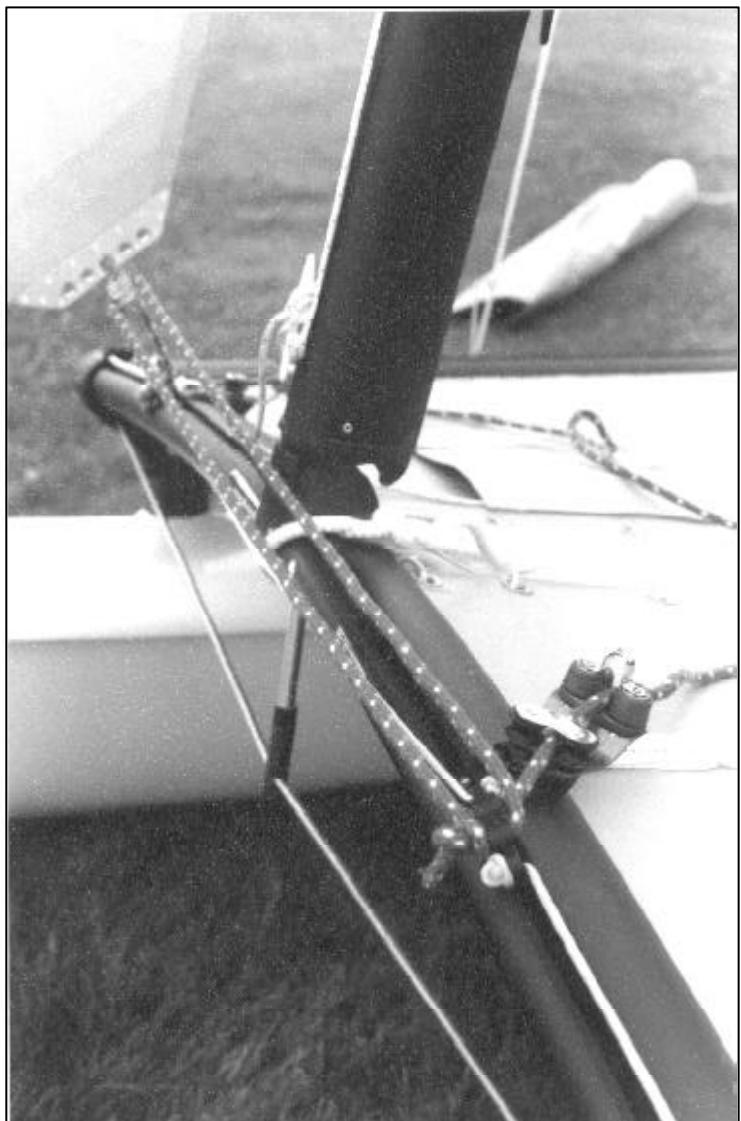
**Attach the righting line to one of the front pylon with a figure eight knot. Tie the other end to the opposite pylon. The line should be lead under the trampoline through the center lacing.**
