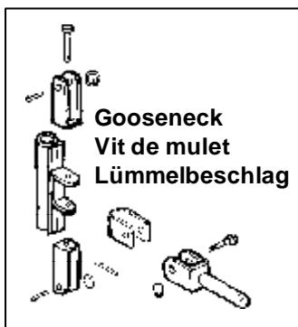
Take the gooseneck and fix it to the grommet of the sail (at the clew). The sheave is facing down. Feed the gooseneck slider in the opening of the mast and pull it down in the gorge.
