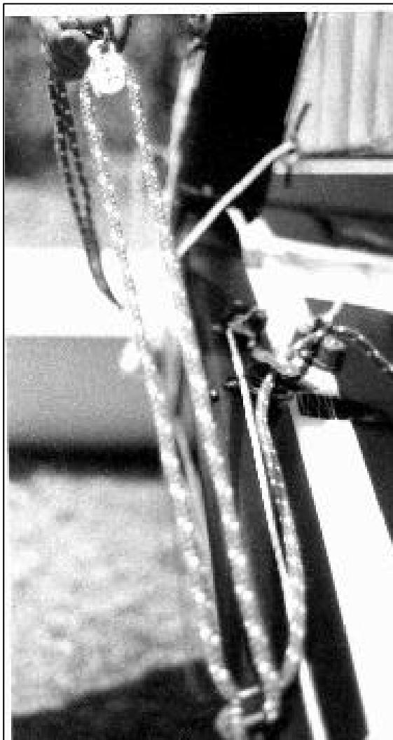
**Lead the jib sheet to one of the clew blocks and back through the second hole of the Trentec traveller car, then back to the jib block on the front crossbar, leading it first through the sheaves and then under the strap of the cam cleat.**
