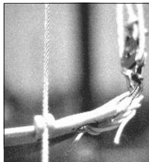
**Secure the plastic hank to the forestay by twisting it 90° onto the wire and hoist the jib. Secure the jib halyard at the bottom of the mast and stow the excess line.**
