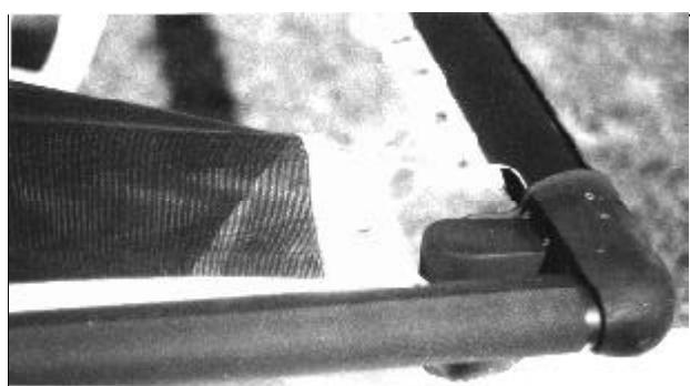
Tie each aft lacing line to the aft corner casting as follows : Start with an 8 knot at one end of the line which you will block into the inferior hole of the rear casting (behind the crossbar fitting). Then, pass the line through the grommet on the side of the trampoline (from underneath), then in the rear trampoline strip (from above). After 3 or 4 laces, temporarily tie it at the aft end. Repeat the same operation for the other side.
